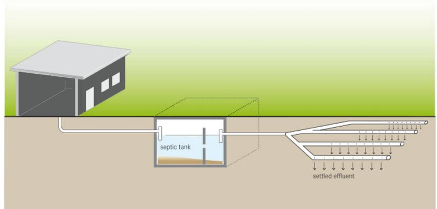
The leaching field further treats the wastewater. If the scum layer overflows the septic tank outlet, the leaching field may quickly become fouled with fats and greases, plugging it, eventually requiring replacement.
